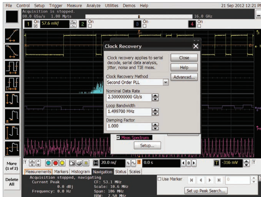
Figure 27. You can choose constant-frequency or phase-locked loop (PLL) clock recovery. With PLL clock recovery, the data rate, loop bandwidth and damping factor are adjustable.
